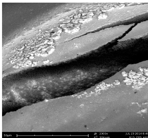
Fig. 9.Polystyrene/amine resin showing breakage and interior loading.
